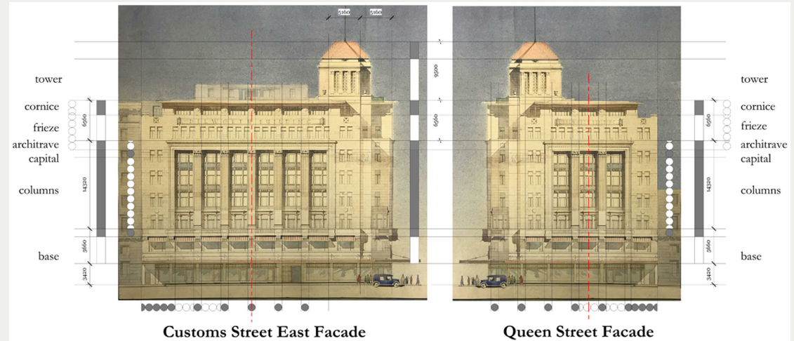
Figure 11. Analysis of the Dilworth Building's façades. Image: Cameron Moore
